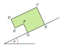
**b** Find, in degrees to 1 decimal place, the greatest value of  $\theta$  for which the lamina can rest in equilibrium without toppling.
