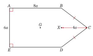
The figure shows a uniform lamina *ABCDE* such that *ABDE* is a rectangle, BC = CD, AB = 8a and AE = 6a. The point X is the mid-point of *BD* and XC = 4a. The centre of mass of the lamina is at *G*.
