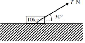
The figure above shows a small box of mass of 10kg, pulled by a rope inclined at  $30^{\circ}$  to the horizontal, along rough horizontal ground
