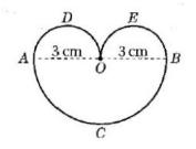
ACB is a semicircle of radius 3 cm, centre O. ADO and BEO are both semicircles of radius 1.5 cm. Find the position of the centre of mass of the framework. 9. Four particles P, Q, R and S of masses 3 kg, 5 kg, 2 kg and 4 kg are placed at the points (1, 6), (−1, 5), (2, −3) and (−1, −4) respectively. Find the coordinates of the centre of mass of the particles.
